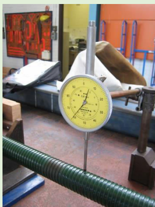
PHOTO C: Measuring deformation of jacks
