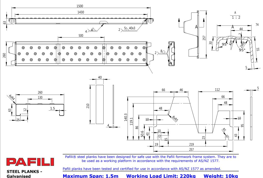
Galvanised Structural Steel aximum Span: 1.5mWorking Load Limit: 220kgWeight: 10kgPAFILI SCAFFOLDINGABN 38002868199phone: (02) 9758 1655www.pafili.com.auinfo@pafili.com.au
