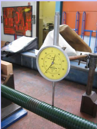
PHOTO C: Measuring deformation of jacks
