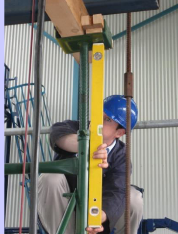
PHOTO B: Measuring effect of load application
