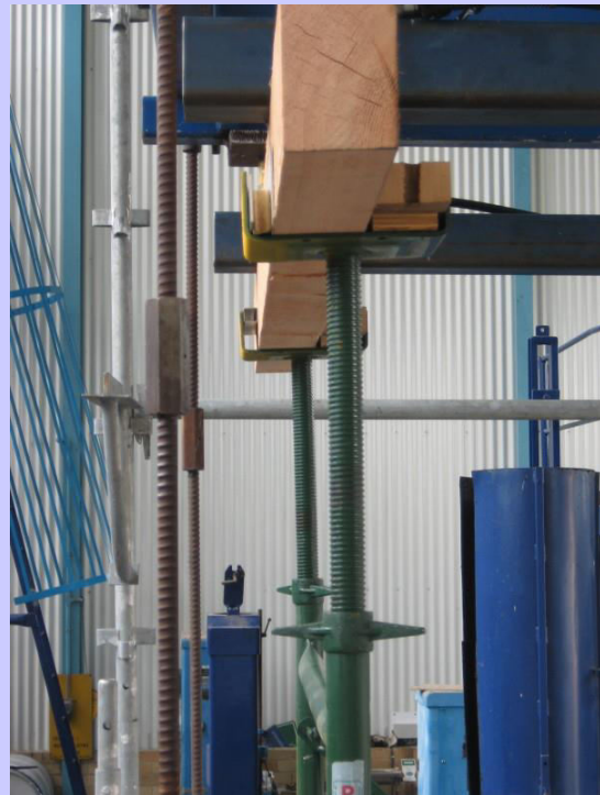
PHOTO D: Eccentric detail under load for Test Arrangement No.2 set-up (Load beams parallel to frames)
