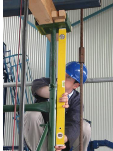
PHOTO B: Measuring effect of load application
