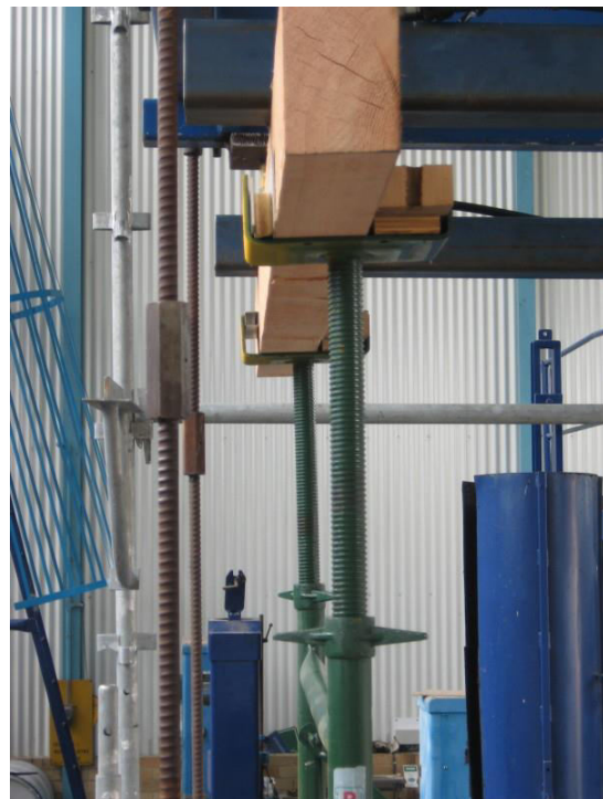
PHOTO D: Eccentric detail under load for Test Arrangement set-up (Load beams parallel to frames)
