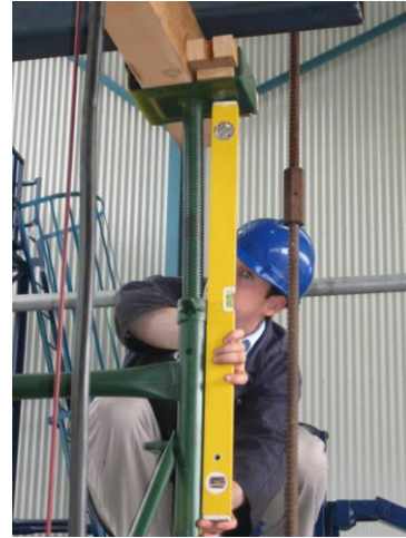
PHOTO B: Measuring effect of load application
