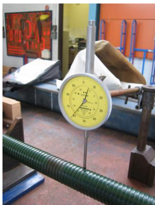
PHOTO C: Measuring deformation of jacks
