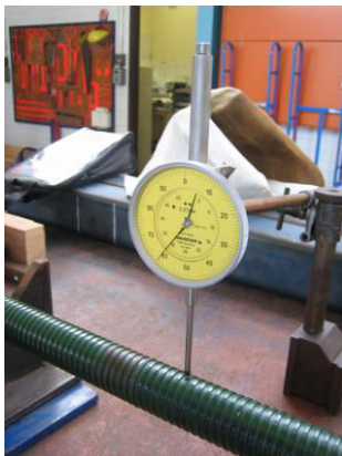
PHOTO C: Measuring deformation of jacks
