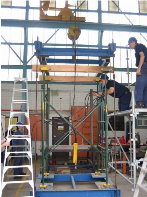
PHOTO A: Test Arrangement No.1 set-up (Load beams perpendicular to frames)
