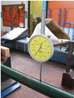
PHOTO C: Measuring deformation of jacks
